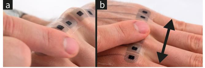
Figure 3: Interaction on challenging, highly curved skeletal landmarks: (a) tapping the peaks and valleys for discrete input; (b) sliding along the knuckles for continuous input.
