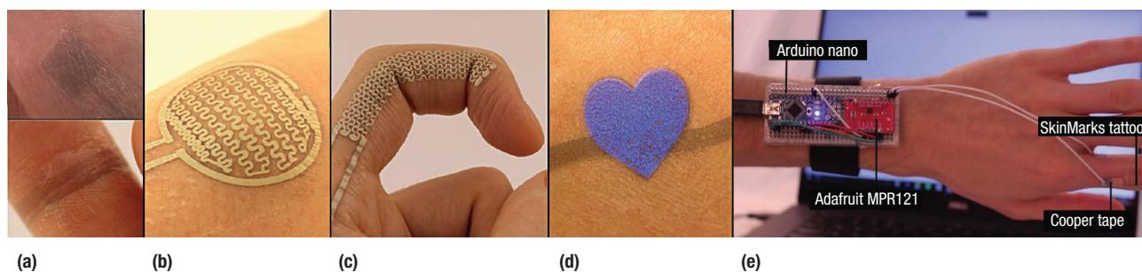
**FIGURE 2.** SkinMarks sensor and display types: (a) capacitive touch buttons and sliders, (b) squeeze sensors, (c) bend sensors, and (d) electroluminescent displays. (e) In our prototypes, the interactive tattoo is wired to a body-worn microcontroller.
