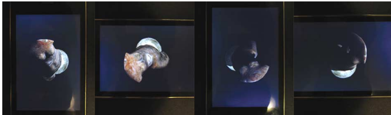
Figure 5. Light source is fixed relative to earth's magnetic pole. Rotating and tilting the device allows different parts to be illuminated by the world-stabilized light source.
