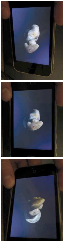
Figure 3. The mobile phantogram uses anamorphic rendering to realistically adapt the viewpoint as the mobile device is tilted.
