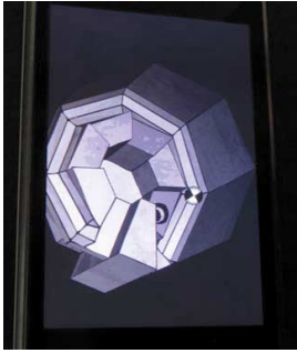
Figure 1. The Diorama game uses phantogram techniques such that not only the game elements are affected when the device is tilted, but also the rendered perspective.
