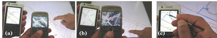
Figure 1. a–b) Multiple mobile devices are wirelessly connected to the surface and provide individual visualizations (road maps and satellite images) of the region indicated by the user’s touch. c) The higher input resolution of the mobile device’s touch screen allows the user to create precise annotations, while also being able to work in a comfortable pose.
