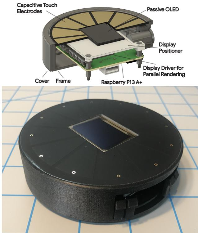
**Figure 4:** Our physical prototype is designed as a compact stack consisting of a Raspberry PI 3 A+ single-board computer, custom PCB with analog DACs, custom passive OLED, and our ring-shaped PCB with electrodes for capacitive touch sensing.
