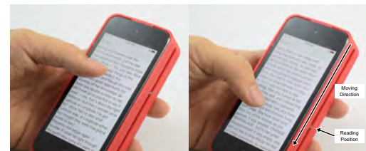
Figure 16: A tactile micro-element represents the current position while scrolling through a document. Touching the element bookmarks the position
