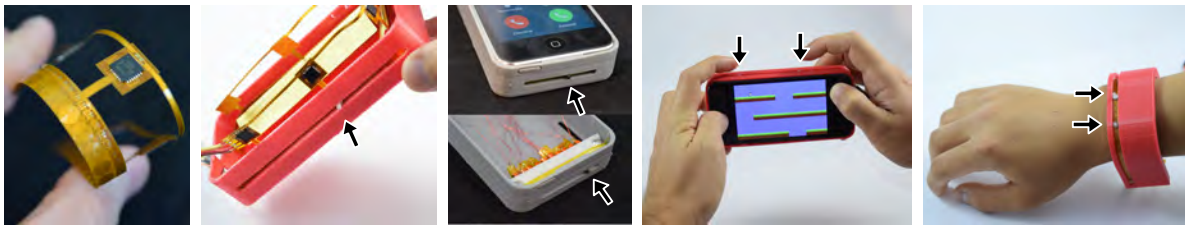
Figure 1: Reconfigurable tactile micro-elements (shown in arrows) for interaction on a mobile device. Left to right: a flexible PCB utilizing micro-coils for magnetic actuation of tactile elements, a mobile prototype using the PCB micro-coil technique, a mobile prototype using low-power switchable permanent magnet actuation, a game played using reconfigurable tactile controls, a wearable band with tactile elements for display and interaction.
