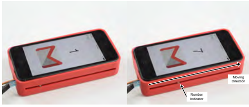
Figure 17: A tactile micro-element changes position based on the number of e-mails available for subtle, tactile notifications.
