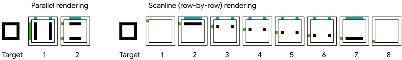
**Figure 2: Parallel rendering activates multiple rows simultaneously to take advantage of redundancies in rectilinear graphics, which can greatly reduce the number of frames needed to render contents. The number of frames needed depend on the content. The Scanline content-agnostic rendering processes each row, which limits the brightness given that at most one row can be illuminated at any given time.**
