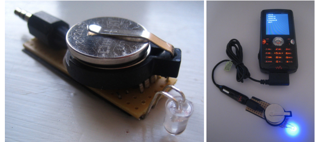
Figure 1. (left) The Auditor consists of a mini stereo connector, resistors, an operational amplifier, batteries and an ultra-bright LED. (right) A cell phone with the Auditor connected to the headphone jack on the handsfree modulates the LED light using software generated audio.
